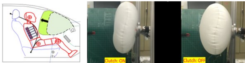
Figure 2. Airbag that would adjust to optimize occupant protection.
