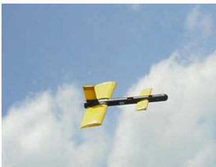
Figure 3: Morphing Inflatable Air Vehicle: (i) with adaptive SMA actuators, (ii) In flight
